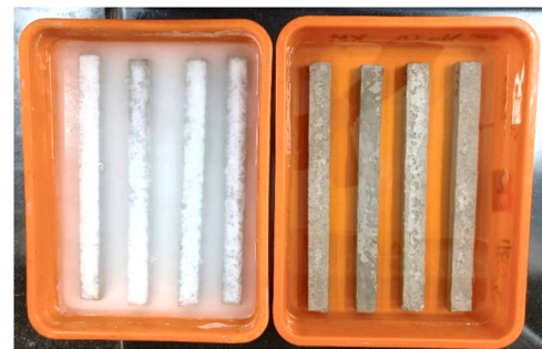
Fig. 5. Photos showing partially carbonated grout specimens immersed in 1 \text{ M Ca(OH)}_2 (shown on the left) and 1 \text{ M Na}_2\text{CO}_3 (shown on the right) solutions.
